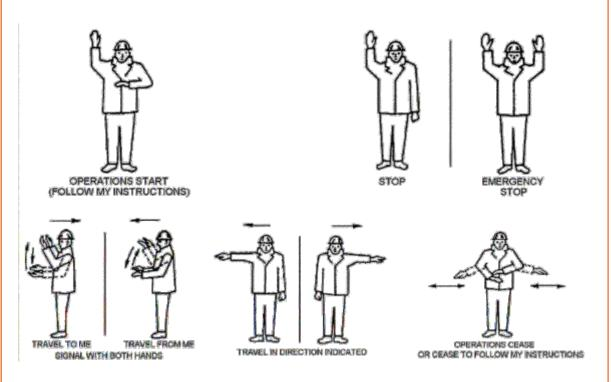
Fig. 3.1.2. Signals To Guide A Mechanic
