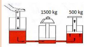
Fig. 1.2.5 (b) Path of the Hydraulic Oil
