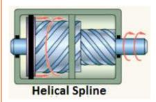
Consists of a cylindrical housing, a shaft and a piston sleeve. Converts linear piston motion into powerful shaft rotation. Helical spline actuators can be employed to actuate ball valves. Both the inside of the piston sleeve and the shaft (where it meets the piston) are splined with matching teeth. The device is hydraulically sealed so that the application of pressure to a port will drive the piston sleeve.
