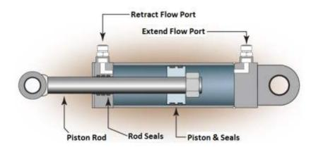
Fig. 1.2.6 (q) Linear Actuator
