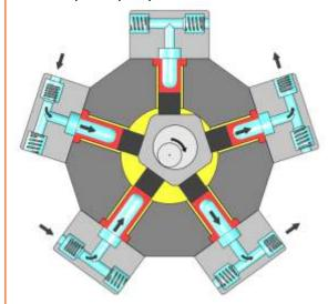
Fig. 1.2.6 (I) Radial Piston Pump
