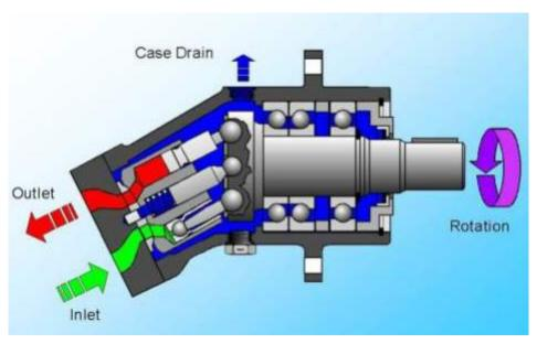
Fig. 1.2.6 (k) Bent-axis Axial Piston Pump
