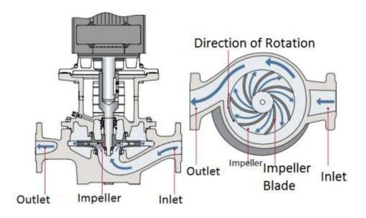
Fig. 1.2.1. How Pump Works
