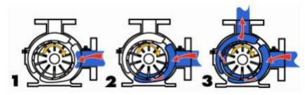
Fig. 1.2.6 (g) Working of Rotary-vane Pump
