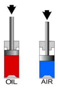
Fig. 1.2.5 (c) Incompressible Hydraulic Fluids
