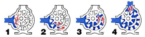
Fig. 1.2.6 (e) Working of Internal Gear Pump
