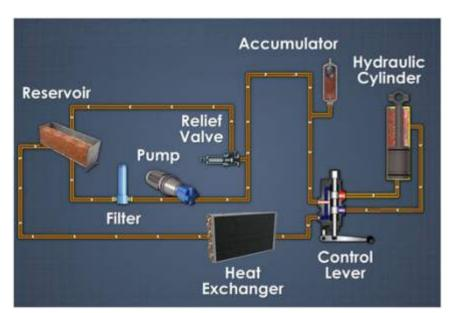
Fig. 1.2.5 (e) Heat Exchanger of Hydraulics
