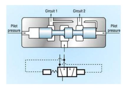
Fig. 1.2.6 (o) Flow Control Valve
