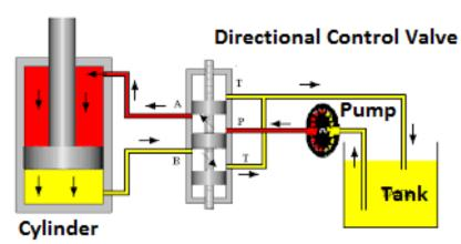
Fig. 1.2.6 (n) Directional Control Valve
