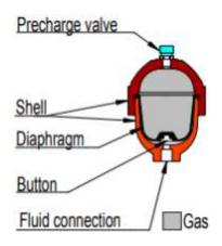
Fig. 1.2.6 (u) Piston and Diaphragm Accumulator
