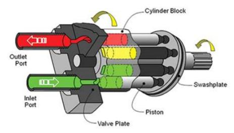
Fig. 1.2.6 (j) Inline Axial Piston Pump
