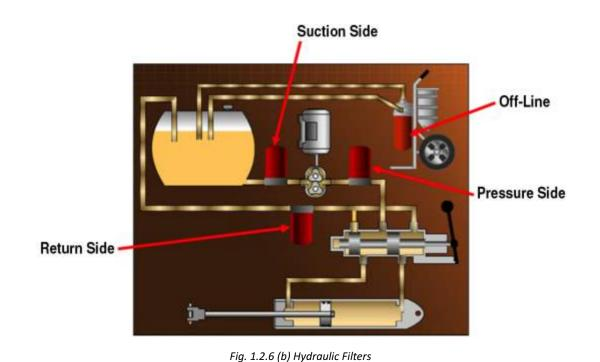
**Suction-side Filters**: These filters protect the pump from contaminants in hydraulic fluid. Generally, they are deployed before the hydraulic pump. Suction-side filters are equipped with wire screen, a higher micron-rating filtering system.
