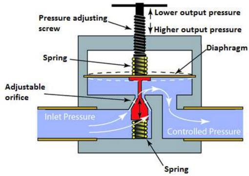
Fig. 1.2.6 (p) Pressure Control Valve
