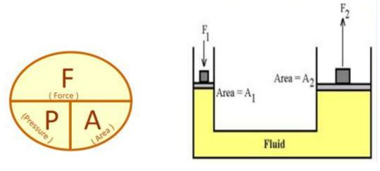
Fig. 1.2.5 (f) Pressure in Hydraulics
